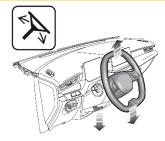
Fully release the locking lever, the steering wheel can be adjusted in 2 directions.
