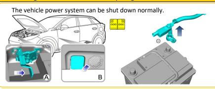
From the inside of the vehicle, pull the bonnet release handle(B), Move the safety catch release handle on the bonnet lock assembly in the direction of the arrow (A) to release the bonnet.
