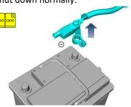
Power off and disconnect the negative cable of 12V low-voltage battery.
