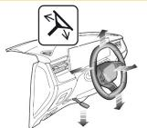
Fully release the locking lever, the steering wheel can be adjusted in 4 directions.
